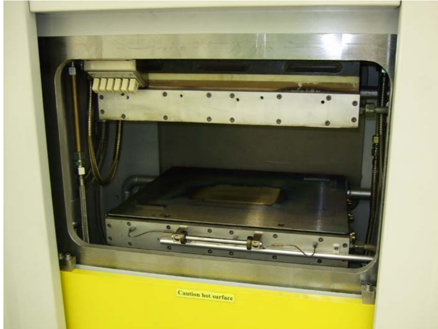
Electrically Heated Hydraulic Vacuum Press for Lamination (Victrex)
